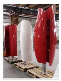
The turbines come in different sizes. The red and white turbines in the illustration are a total of 3 meters high. The turbines are also available in heights of 1 and 6 meters. The black turbine depicted above has blades that are 1 meter high, and the pole height is adjustable.
